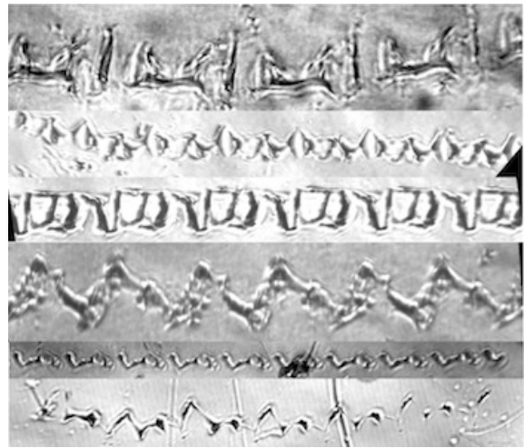
FIG. 12. Different types of “evaporated” regular periodic structure tracks in Polychrome Litho film, no pre-exposure, developed with constant agitation.
