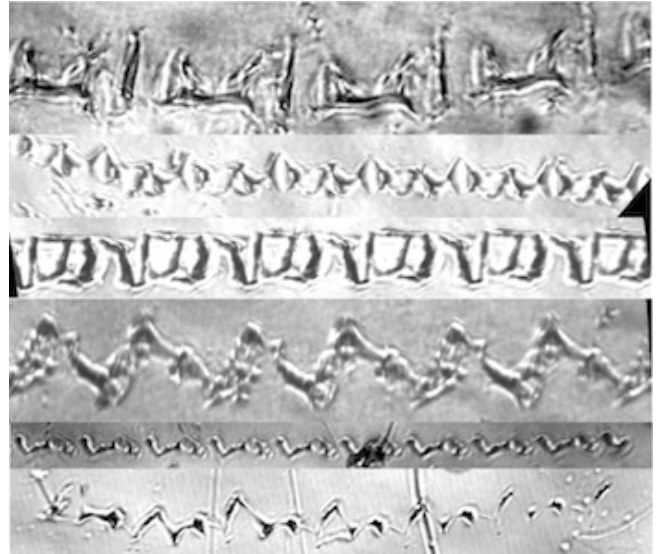
FIG. 14. (3:O) Different types of “evaporated” regular periodic structure tracks in Polychrome Litho film, no pre-exposure, developed with constant agitation.
