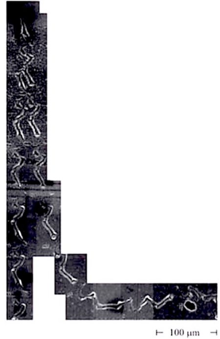
FIG. 67. Adamenko and Vysotskii track evaporated in MDS showing parabolic curvature. Detail of track using high magnification. Note similarity to Fig. 17
