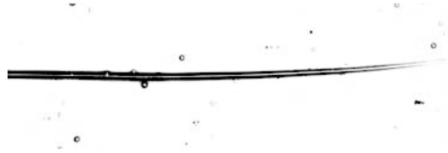
FIG. 12. (1:R) Detail of 69mm track. Track structure of the internal saturated track surrounded by areas of local bleaching can be clearly seen. Each end of the track “fades,” that is, the density of the central track image fades into the background as the local bleaching decreases and the track width decreases as well.
