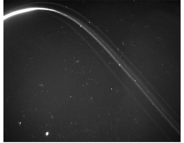
FIG. 31. (2:O) bundle one Track appears to be splitting into sub-tracks. Micrograph at 7x magnification. Kodolith Ortho type III film using permanent magnet M1.
