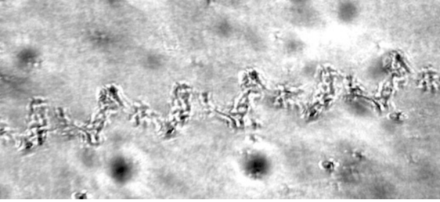
FIG. 16. (3:O) zigzag Exposure shows a periodic evaporated track in the form of a saw tooth at 400x magnification.
